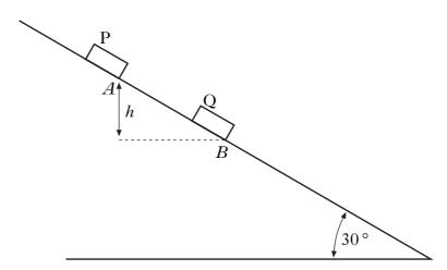
When block P is released, it slides down the ramp colliding and coupling with block Q. The combined blocks then move down the rough section of the ramp, coming to rest at a vertical height  $\frac{1}{2}h$  metres below B.
