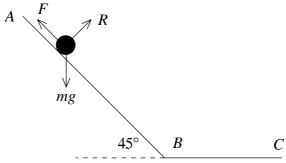
(a) Resolving perpendicular to the chute gives  $R = \frac{1}{\sqrt{2}}mg$  so
