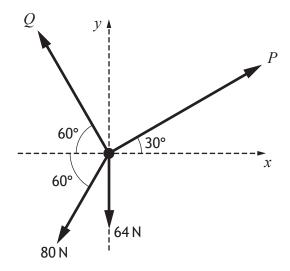
The tensions in the four ropes are P, Q, 80 and 64 newtons respectively, and their directions relative to the axes are shown.
